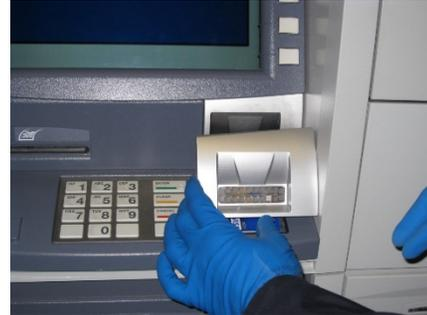
**How it works:** A credit card skimmer is a portable card-reading device that is attached within the legitimate scanner, capturing your card's information when you swipe or insert it. Cameras and/or keypad recorders may also be used in card skimming plots. With your debit card information and personal identification number (PIN), thieves have the information they need to make unauthorized purchases and possibly drain your account.
